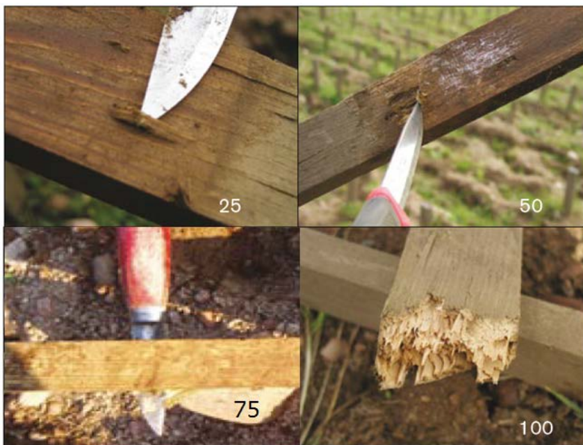
Figure 7 Rot index visualisation in compliance with the European field testing standard EN 252, used for analysing the degradation of timber in ground contact. (Reference: Råberg, Terziev 2006)
