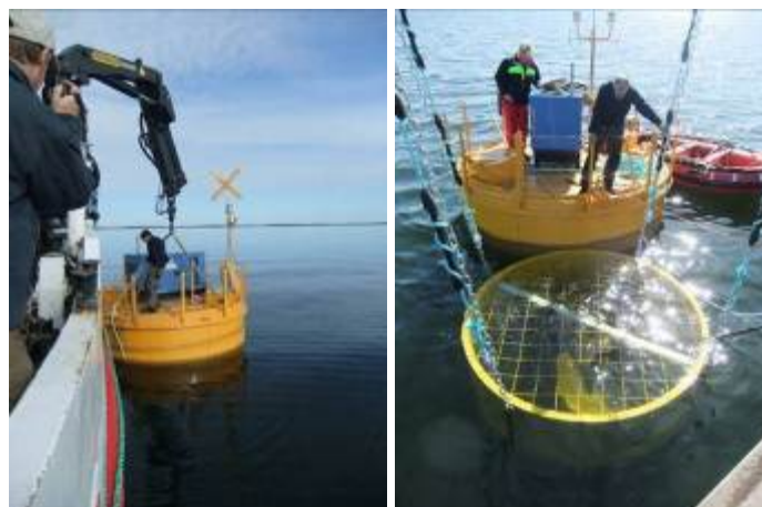
Figure 3.2. Launching of the main float and the pump-house.
