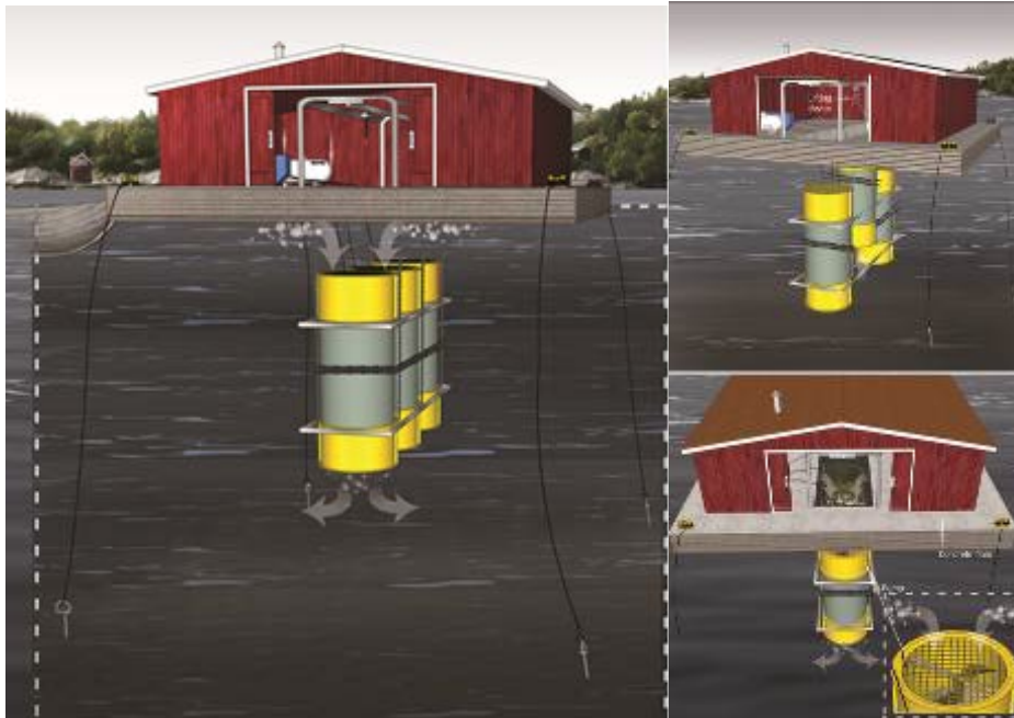
Figure 3.13. Concept of a possible full-scale application and design of WEBAP II - Electric oxygen pump with three pumps in combination.
