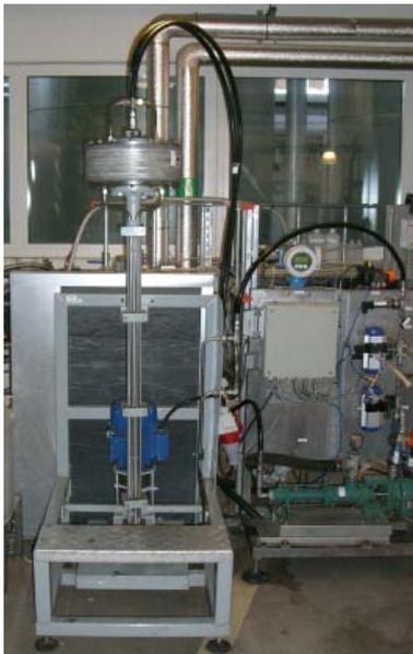
**Figure 11: VSEP unit (membrane stack and electrical engine)<sup>1</sup>.**
