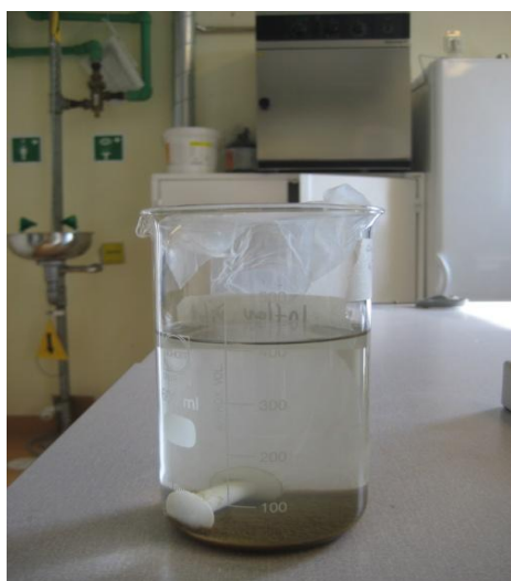
Fig 9. KMnO_4 treatment for 4 hours followed by Mg-Ca flocculation.
