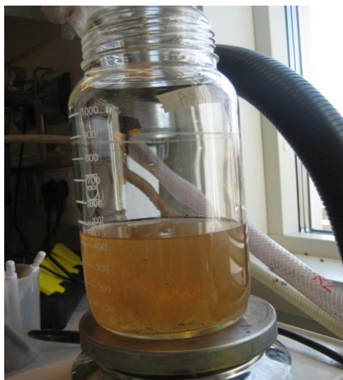
Fig. 7. The process of concurrent treatment of \text{KMnO}_4 and Mg-Ca flocculation
