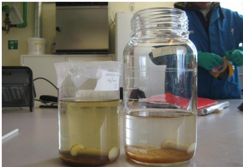
Fig. 8. Left: KMnO_4 treatment for 4 hours. Right: Concurrent treatment of KMnO_4 and Mg-Ca flocculation.
